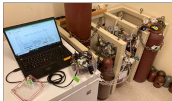
Calibration set up: 3 gas standards measured (0 ppm, 200 ppm, 400 ppm CO 2 )
