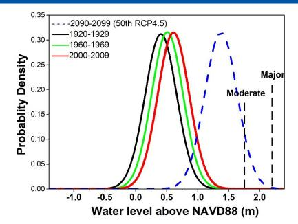
Illustration of how the probability of water levels exceeding National Weather Service flood thresholds (moderate and major) increases with sea level rise. This could lead to an exponential increase in surge barrier closures. Probability density functions are based on historical water level data from The Battery, NYC, with the 50th percentile regional sea level rise projections to 2090-2099 for a moderate emissions pathway (RCP 4.5) (Chen et al., submitted 2020).
