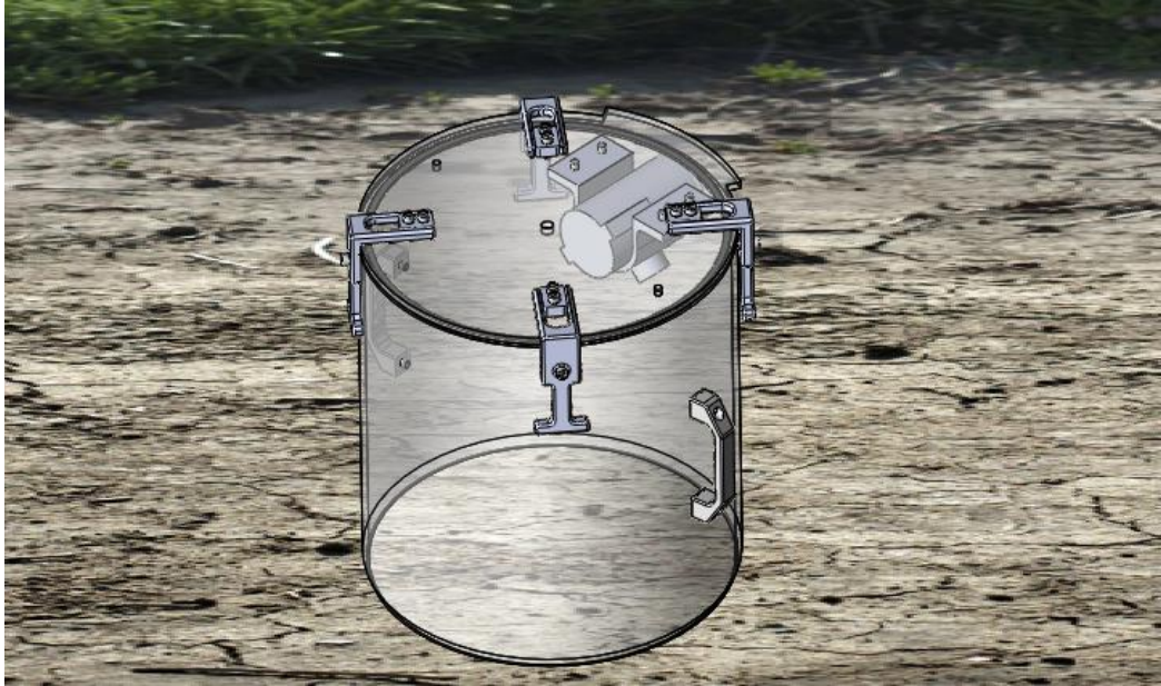
Figure 12. The benthic chambers design shown in Solidworks CAD displays the beveled edge at the bottom of the design to allow for the midsection to easily be buried in the sediment for testing.
