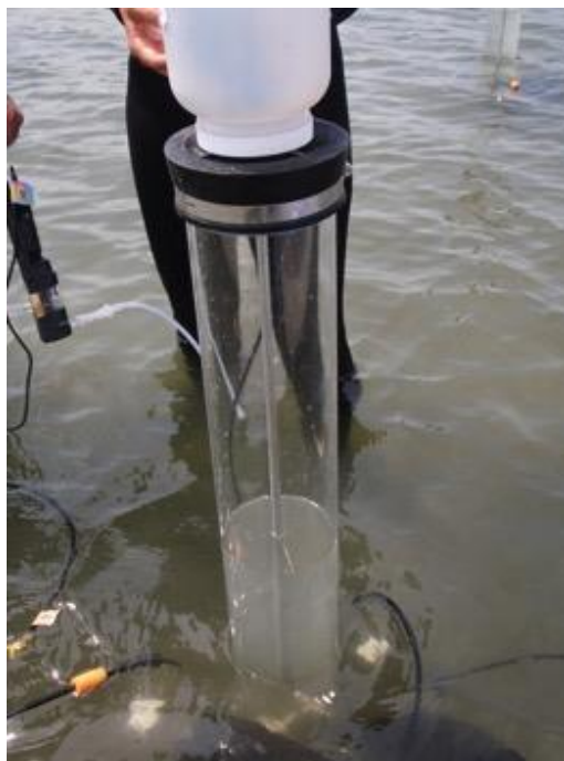
Figure 3. Clear acrylic cores were powered with a hand drill in a bottle and had a diameter of 13.3 cm.
