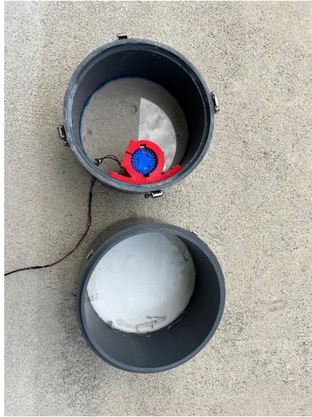
Figure 7. The top view of the benthic chambers in an unlatched configuration was shown. A custom 3D printed mount was created to attach the bilge pump to the midsection. The white polyethylene plate was also shown in the sampling base, and the polycarbonate lid on the midsection.
