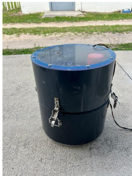
Figure 6. The initial prototype was manufactured and tested to determine the effectiveness of the design. The benthic chamber can be seen in an operational configuration, with latches aligned to secure the midsection and the sampling base.
