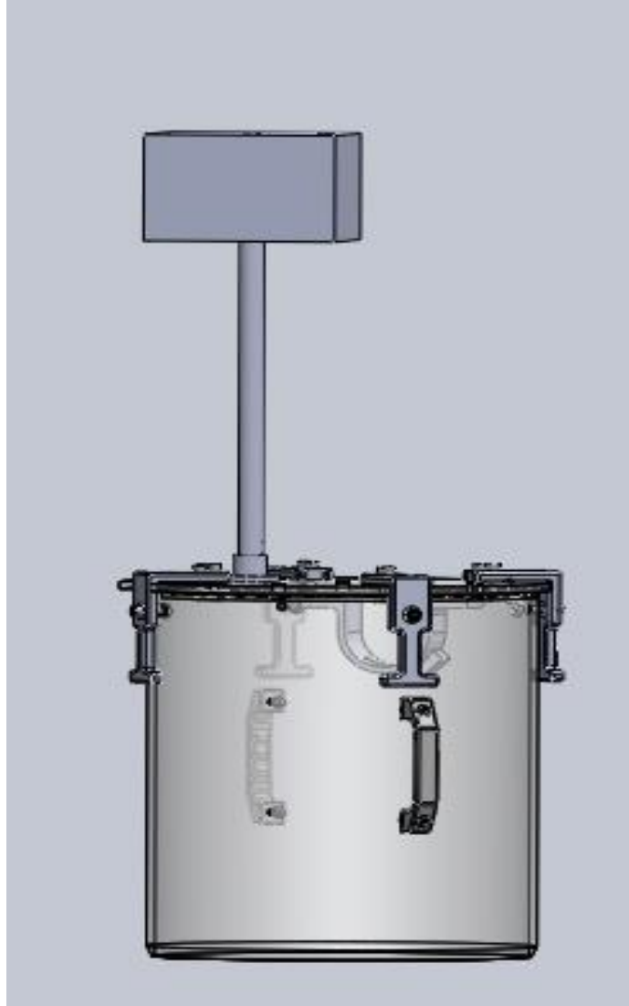
Figure 30. Battery support concept design.
