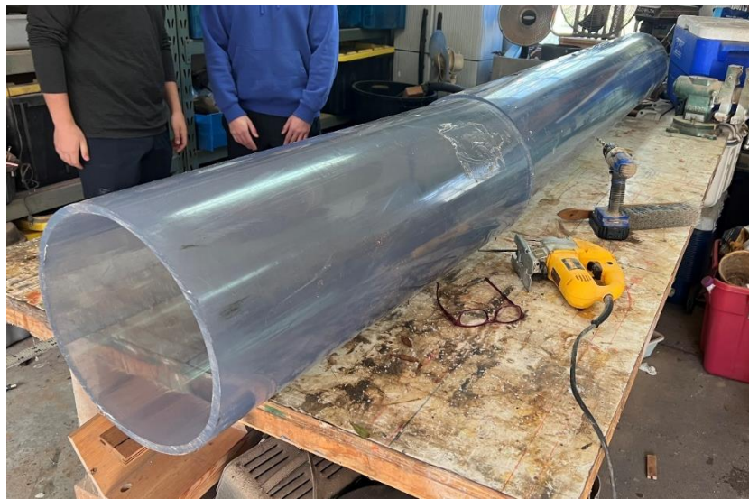
Figure 16. The clear PVC arrived in a 10-foot section, and had to be cut down to have size, which was performed by a hand-held reciprocating saw.
