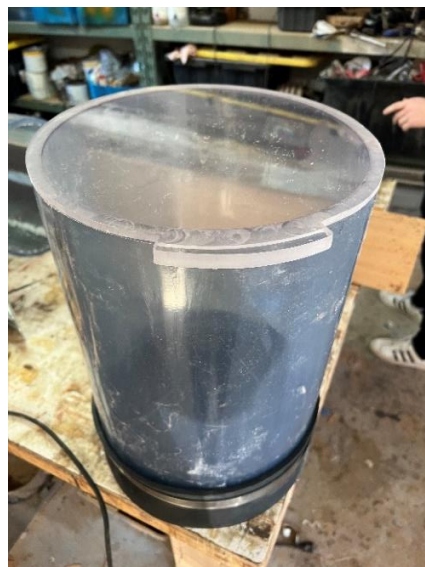
Figure 18. After the midsection was cut from the PVC material, and the lid from the polycarbonate material, these pieces were assembled together to determine the quality of the fit for the overall assembly.
