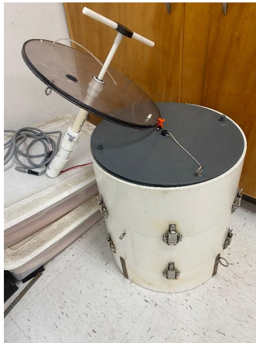
Figure 4. The 12-inch diameter PVC benthic chamber can be observed, with two-midsections and a sampling base.
