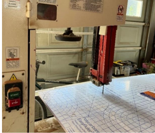
Figure 17. The Grizzly band saw was used to cut a defined shape of the lid.
