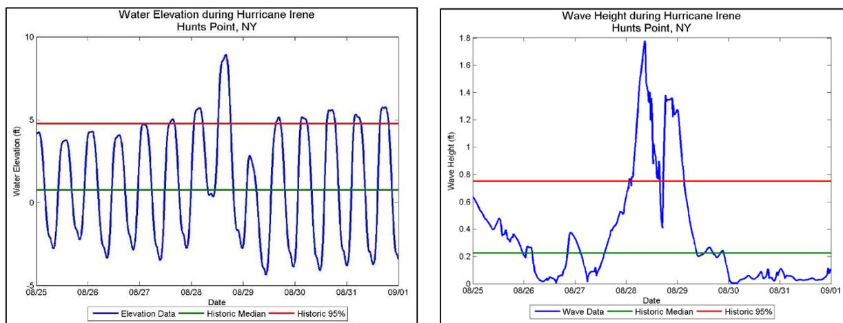
Figure 9 - Example water level and wave height hindcasts during Hurricane Irene
