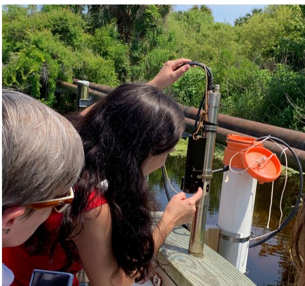
Left: Project team members, Jenna Reimer and Dr. Shirley Baker, checking the nitrate sensor at the Mickler's Weir.
