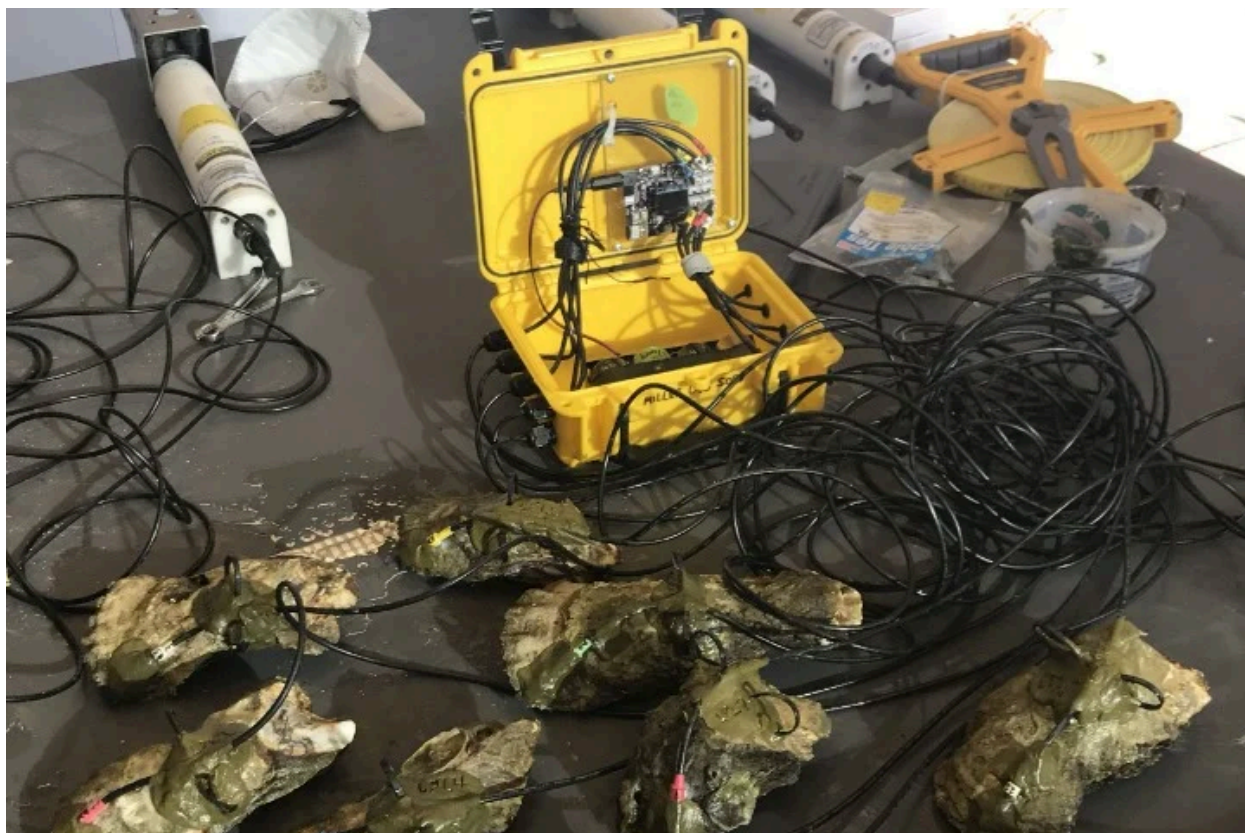
Caption: Biosentinel oysters ( Crassostrea gigas ) attached to a data logger prior to deployment.
