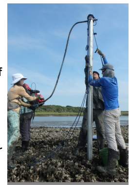
Jaleigh and crew using a vibracore to collect the core sample.
