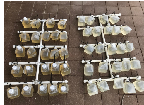
Top (L-R): Justina holding cubitainer. Justina adding treatments to cubitainers. Center (L-R): Collected cubitainers. Deployed cubitainers. Bottom: Cubitainers attached to PVC pole deployment system
