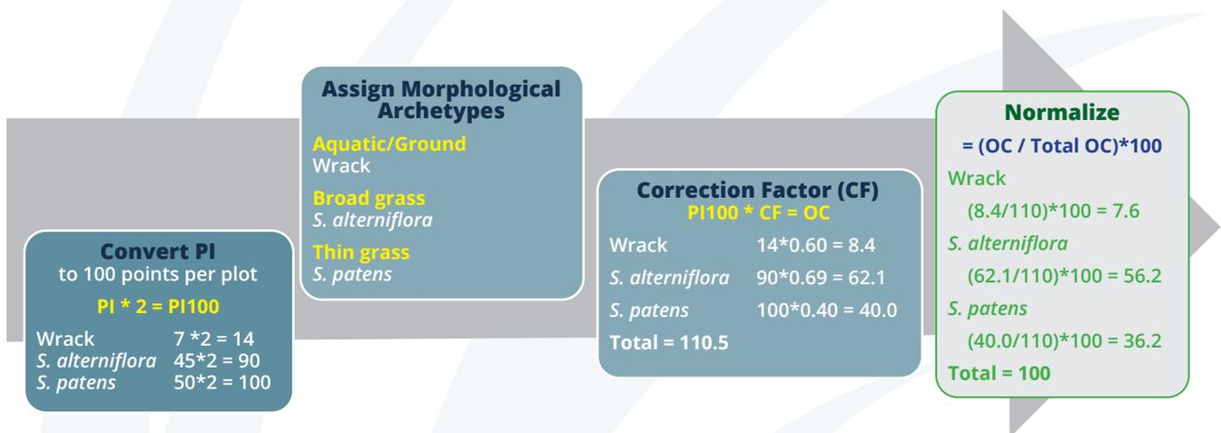
Example data shown above is from a 50-point plot in a 1m<sup>2</sup> quadrat.
