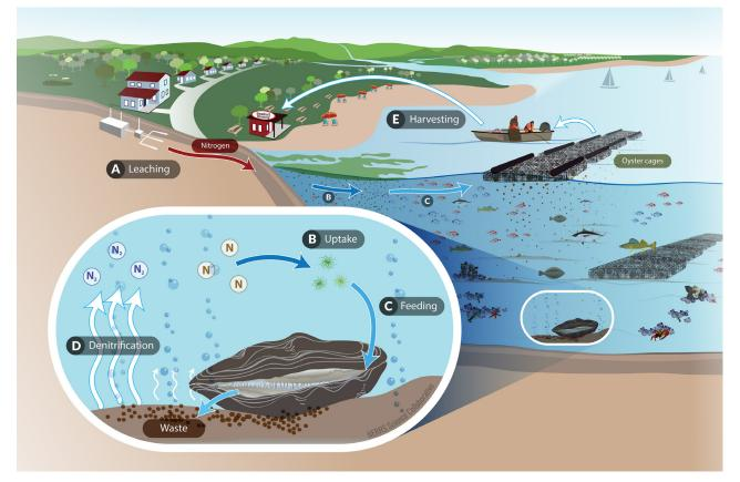
This graphic helps explain how nitrogen gets into coastal waters, and how oysters can help remove nitrogen by stimulating denitrification in the sediment and through the harvesting of oysters for food.
