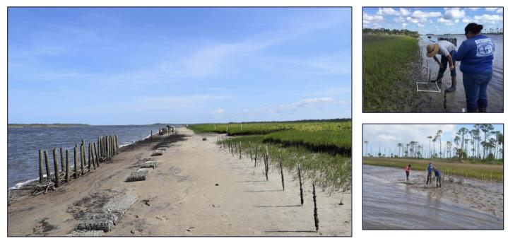
Figure 17: Photograph showing full experimental setup and monitoring structures. PVC poles on the right mark the initial shoreline position and the spots selected for ecological monitoring.
