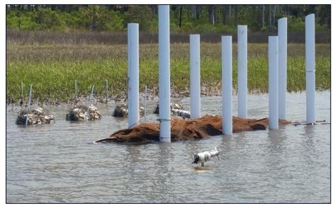
Figure 25: Pilot site gabion breakwall with wave energy gauge
