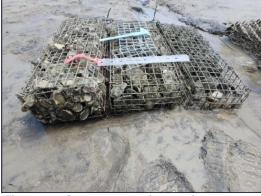
Figure 18: Oyster measuring equipment on three small oyster gabions
