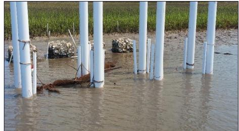
Figure 16: Branches missing from the pilot site; likely missing due to wave energy
