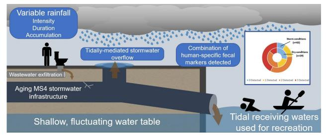
This figure illustrates key findings about how wastewater is contaminating stormwater and affecting coastal waters (credit: Hart et al. 2020. Science of The Total Environment, DOI: doi.org/10.1016/j.scitotenv.2020.141124)
