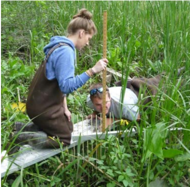
Figure 2. SET apparatus installed and observer taking measurement with meter stick atop the SET arm (photo credit Hudson River NERR).
