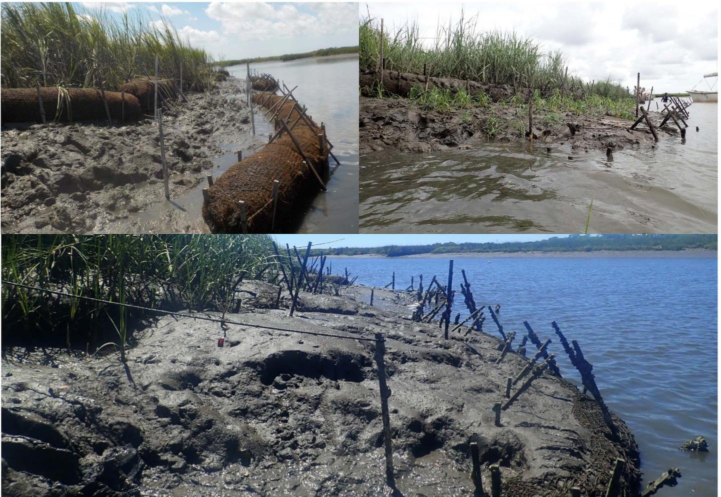
**Figure 3.17.** Double-row coir log treatment at Orangegrove Creek in August 2017 (upper left), May 2018 (upper right), and April 2019 (lower). The upper left coir log went missing at some point between August 2018 and April 2019.
