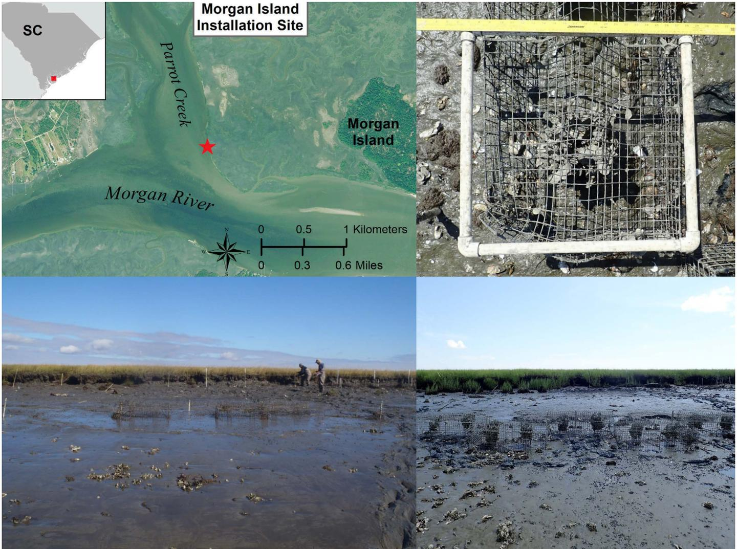
**Figure 3.12.** Aerial view of the living shoreline research site on Morgan Island Creek (upper left). Two MWR units were dislodged and relocated nearby by Hurricane Matthew (lower left) but were easily moved back into position. Live oyster coverage on MWR in August 2018 (upper and lower right).
