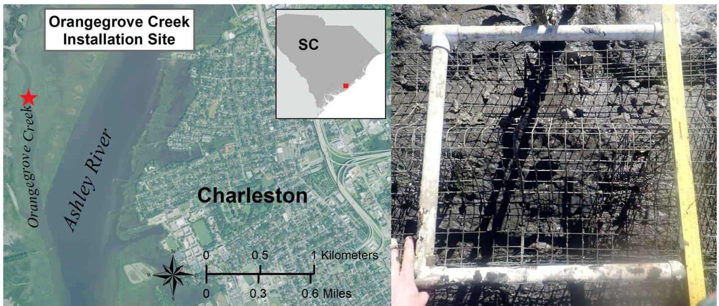
**Figure 3.11.** Living shoreline research site on Orangegrove Creek with an aerial view (left). Live oyster coverage on MWR at Orangegrove Creek in April 2019 (right) with limited recruitment and growth after 21 months.
