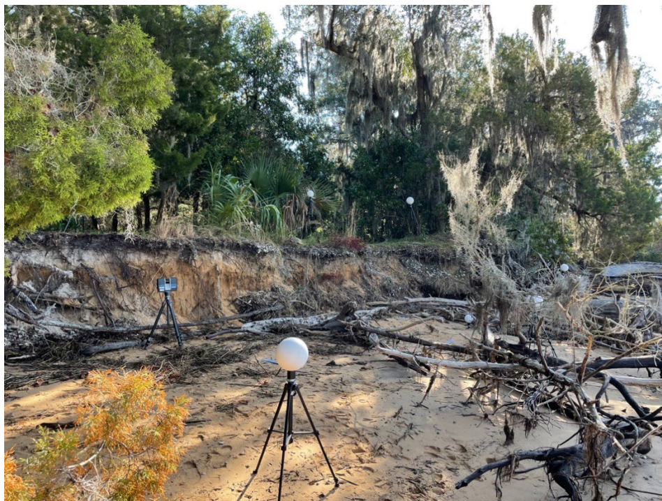
Figure 7 Terrestrial laser scanning at Wright's Landing using a Faro Focus 350s, target spheres, and calibrated scale bars.
