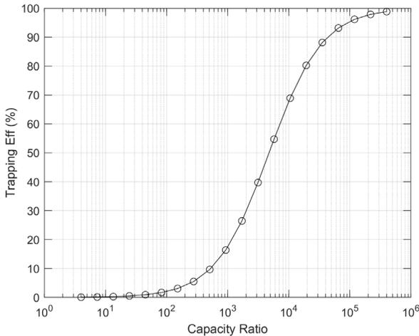
**Figure 2** – Impoundment trapping efficiency ( $TE$ ) for different capacity ratios ( $C/W$ ) estimates the percentage of transported sediment that is trapped within an impoundment from Brown (1943). Capacity ratio is water volume or capacity in units of  $\text{m}^3$  by watershed area in  $\text{km}^2$ .
