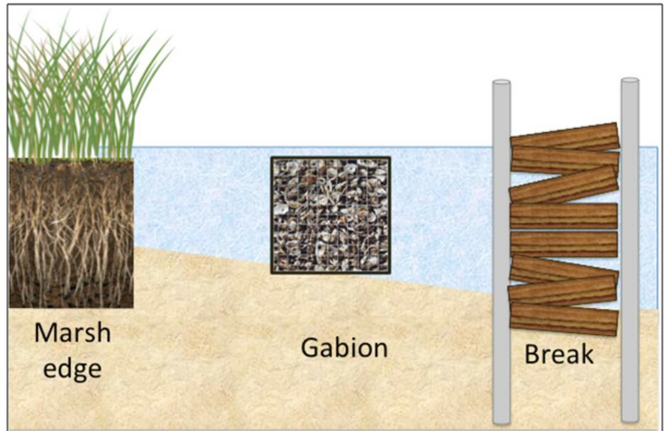
An in-depth study monitored boat wake and wave energy, oyster reef development, and salt marsh edge movement to evaluate the effectiveness of the gabion-breaks in protecting and enhancing coastal habitat in areas with high boat traffic. The project team incorporated findings into training activities for restoration practitioners and coastal managers and interpretive exhibits for reserve visitors.
