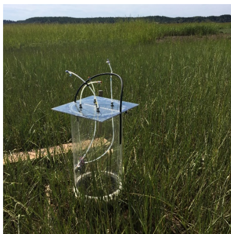
Fig. 1. The transparent chamber used for \text{CO}_2 and \text{CH}_4 measurement.
